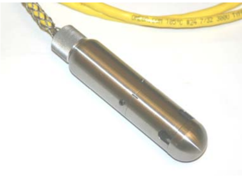
5 in. long by 1.25 in. diameter Thermal Probe with four infrared sensors
